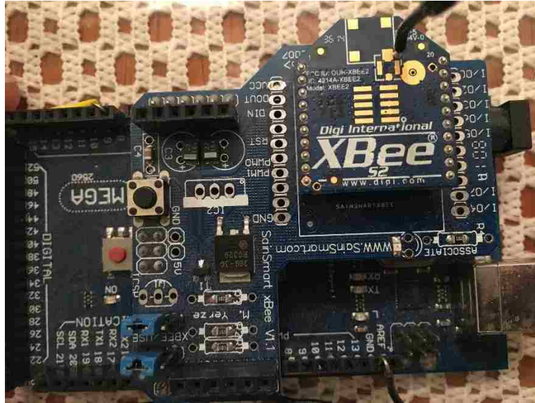
Figure 24: XBee Module Connected to The XBee Shield
