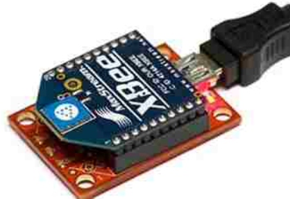
Figure 13: XBee Explorer Connected to XBee module
